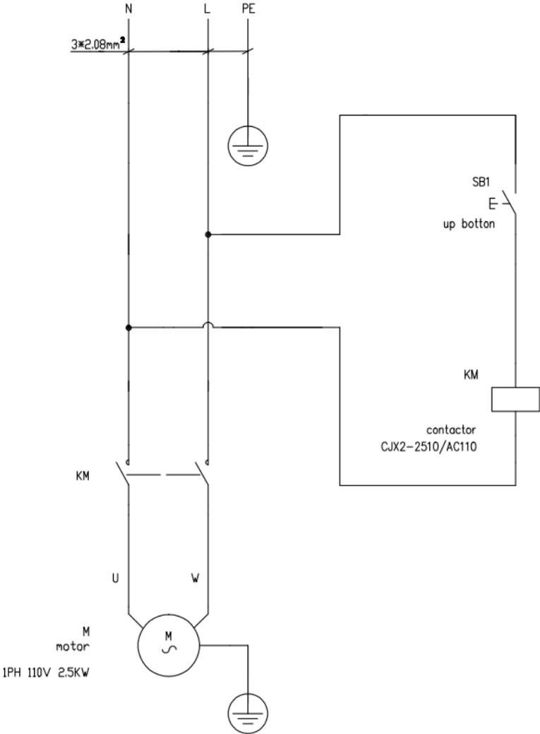
Annex 5, Separate diagrams for the lift
