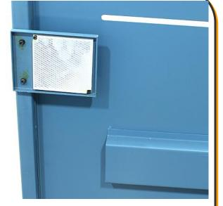
The emitter bounces a laser light beam off of the reflector and back to the emitter to close the circuit and allow the shear to operate.
