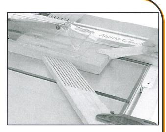
9. Connect the saw to the power source, turn it ON, and allow it to reach full speed.
