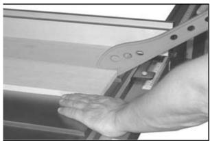
WARNING: Serious injury can be caused by kickback. Kickback is a high-speed ejection of stock from the table saw toward an operator. The operator or bystanders may be struck by flying stock, or the operator's hands can be pulled into the blade during the kickback.
