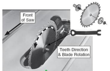
loosen and remove the arbor nut, flange, and blade.
