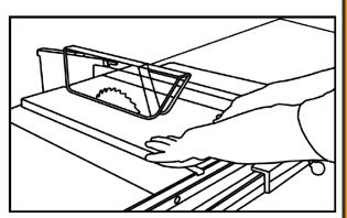
by the blade) from closing and binding the blade, which can overload and/or stall the motor or cause the blade to lift and eject the workpiece towards the front of the saw at very high speeds. The blade guard keeps your fingers away from the blade and also reduces the amount of sawdust flying free.
