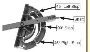
To use a setting other than 90°, loosen the lock knob (A) by turning it counter-clockwise, pull the stop-lock pin (B) and rotate the miter head to 45°, or any angle shown on the numerical guide.
