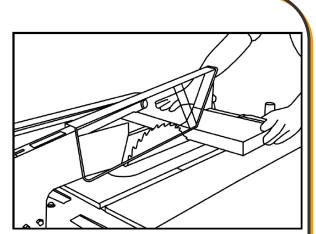
Place the work stock against the miter gauge and
