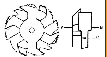
The dado head set is assembled to the saw arbor in the same manner as the standard saw blade.
