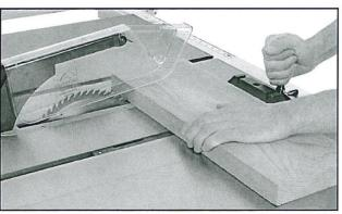
WARNING: Turn OFF the saw and allow the blade to come to a complete stop before removing the cut-off piece. Failure to follow this warning could result in serious personal injury.
