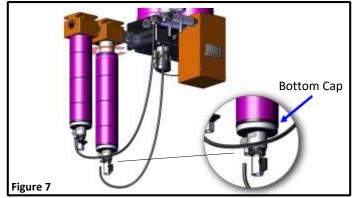
Release system pressure in the dryer, open either ball valve located on the bottom of the filter housing to verify there is no pressure remaining inside the unit. *Figure 7 Note: When performing maintenance on a tank mounted dryer, either put the dryer into hypers made (news 2) or release of a tank*
