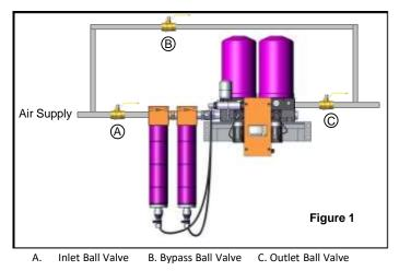
Using the Dryer: Open the inlet (A) and outlet (C) ball valves and close the Bypass (B) ball valve to direct air flow through the regenerative dryer. This will provide clean, dry air downstream.
