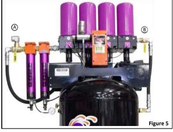
A. 3-Way Inlet/Bypass Ball Valve
