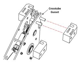
Top View. Drawing shows how to properly install two install Slide Blocks onto the Crosstube Gusset.
