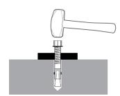
The Expansion Sleeve of the Anchor Bolt may prevent the Anchor Bolt from passing through the hole in the Base Plate; this is normal. The hammer or mallet will get the Expansion Sleeve through the Base Plate and into the hole.
