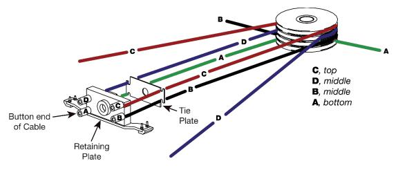
11. Near the Hydraulic Cylinder, loosen the Retainer Plate enough to give you room to slip the Button End of each Cable into its spot on the Tie Plate.
