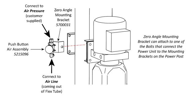
Drawing shows the Pushbutton Air Valve Assembly and its connections to the Mounting Bracket on the Power Post. Not all components shown. Sample Power Unit shown.
