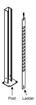
So how do the Runways come down if the Safety Locks are engaged? To lower the Runways, you raise them a few inches (to get them off the Safety Locks), then press and hold down the pushbutton on the Pushbutton Air Valve. While you hold down the pushbutton, the Safety Locks are moved away from the Ladders; in this position, they cannot engage, which allows the Runways to be lowered.
