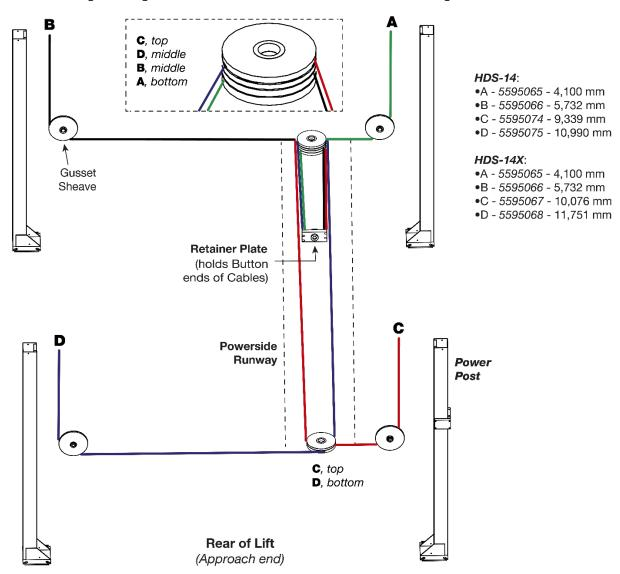
The following illustration shows the Cable Sheave Pairings underneath the Powerside Runway. *Lubricate the Cable Sheave Pins and Bores with Red Lithium Grease.*
