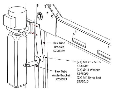
BendPak recommends orienting the Flex Tube so that the lines coming out of it are near where it connects on the Power Unit and to the Pushbutton Air Valve.
