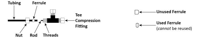
**NOTICE**: *Ferrules can only be tightened once*. When you tighten the Nut on the Threads, the Ferrule gets compressed; it literally changes shape and *cannot* be used again.
