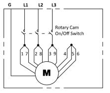
Rotary Cam On/Off Switch
