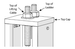
Drawing shows the Threaded end of the Lifting Cable in position in the Top Cap.
