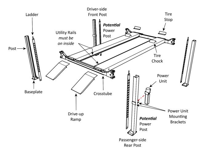
Drawing shows the two possible Power Post locations; only one Post has Mounting Brackets for the Power Unit. Not all components are shown.
