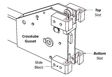
Front View. Drawing shows the Top and Bottom Slots created by the Slide Blocks. Not all components are shown.
