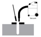
BendPak recommends using a vacuum to clean the hole. You can also use a wire brush, hand pump, or compressed air; just **make sure to thoroughly clean each hole**.
