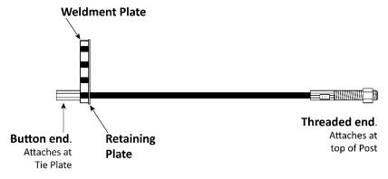
Drawing not to scale. Not all components shown. The Weldment Plate, located under the Powerside Runway, comes attached to the end of the Piston on the Hydraulic Cylinder.
