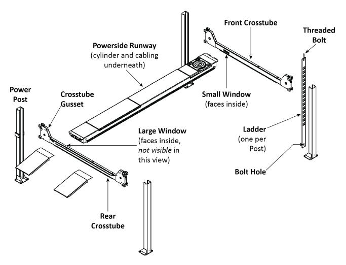
Drawing not necessarily to scale. Some components not shown. Offside Runway removed for clarity. Crosstubes have a Crosstube Gusset on both ends.
