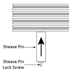
Using a Red Lithium Grease Lubricate each Sheave Pin Prior to inserting through the Sheaves. Figure shows Sheave Pin being pushed up into the four Cable Sheaves at the Rear of the Lift.
