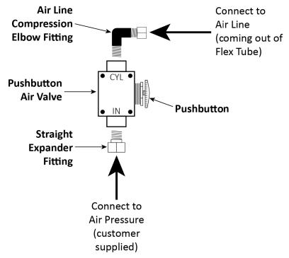
The elbow fitting connects to the opening labelled **CYL**. The straight fitting to the opening labelled **IN**. See the drawing above.
