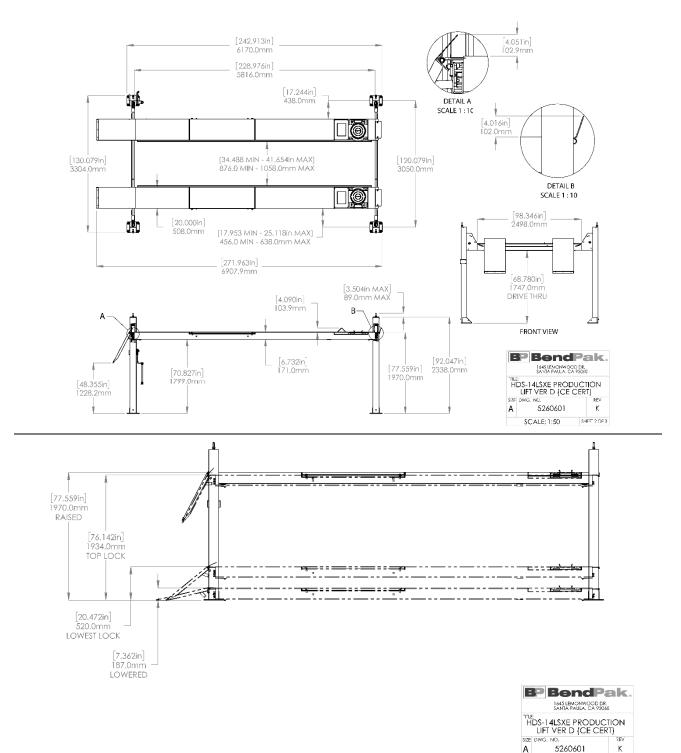
1. DIMENSIONS SHOWN ARE WITH THE LOCK LADDERS ADJUSTED ALL THE WAY UP
