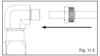
3. Install the 90-degree Hydraulic Fitting in the port at the ram end of the Cylinder. On the pipe thread side of the Fitting it is recommended to use Teflon Tape or pipe sealer. DO NOT USE TEFLON TAPE on the JIC flared end.
