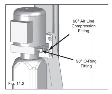
2. Remove the captive nut on the Compression Fitting. Insert the Plastic Air line through the alignment sleeve and into the end of the fitting until it bottoms out. Then tighten the nut on the fitting. (See Fig 11.3)
