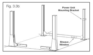
5. With the Columns standing and the cross tubes in position, install the Safety Ladders. Pass the ladders through the Column openings and drop down through the Slide Block guide slots on the Cross Tube until the Ladders come to rest on the Base Plates. **DO NOT BOLT** Columns down at this time. (See Fig. 3.4 - 3.7)
