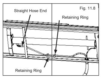
8. Connect the straight end of the Power Unit Hydraulic Line to the 90° Power Unit Fitting. Connect the Return Air Line to the 90° Air Fitting. There will be one air line hose left unconnected at this time. This air line hose will be used to activate the pneumatic safety locks on the next page.
