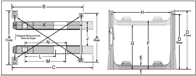
IMPORTANT NOTE: Confirm square layout; diagonal measurements must be equal.
