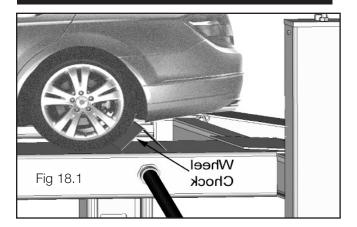
To reduce the risk of property damage, personal injury, or loss of life, NEVER park any vehicle on the Lift's runways without placing two suitable wheel chocks behind each rear tire so that the vehicle cannot roll backward off the Lift. Vehicles parked on Lift MUST also be placed in Park or First Gear (Manual Transmission) with the Parking Brake fully applied.
