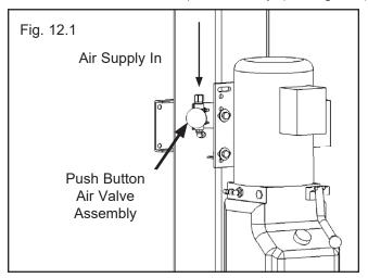
2. Route the air line that was left unconnected in Step 10 to the 90° Air Line Compression Fitting of the Push Button Air Valve Assembly. (See Fig 12.2)
