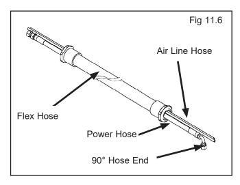
6. Install the end of Flex Hose with the Straight Fitting on the Hydraulic Hose into the hole in the Powerside Runway adjacent to the Power Unit. Install the end of the Flex Hose with the 90° Fitting on the Hydraulic Hose in the Flex Hose Bracket Assy. Tighten the plastic nuts securely.
