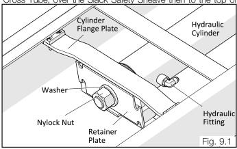
each Column. Secure using the M22 Hex Head Nuts and Flat Washers. Tighten each nut until there is at least one inch of threads protruding through the top of the Nut. The Cables will remain loose until start up and final Cable adjustments are made. (See Fig. 9.2 - 9.3)
